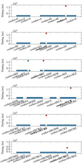
Fig. 13: Bytewise leakage of the secret (S,E,C,R,E,T) from ZRAM. Times for guesses (0-9, A-Z) for each of the bytes are shown. The highest value in each plot (shown in red) indicates the correct secret value for the byte. The standard error is below 1% for all guesses.
