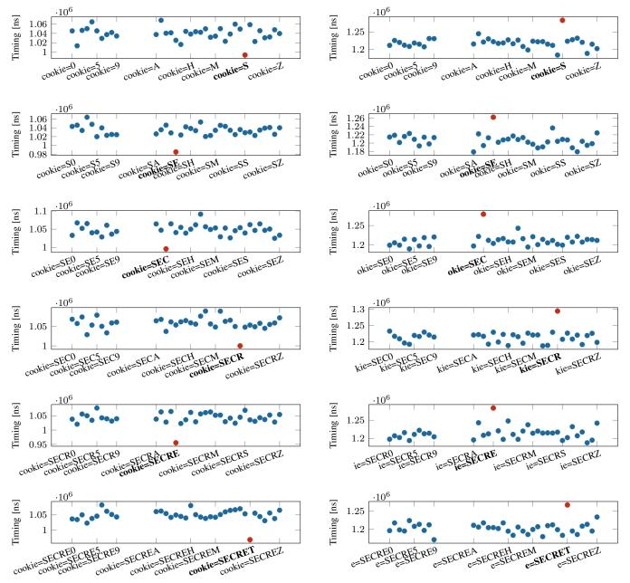
Fig. 11: Bytewise leakage of the secret (S,E,C,R,E,T) from PHP-Memcached. In each plot, the lowest timing (shown in red) indicates the correct guess. The standard error is below  $1\,\%$  for all guesses.
